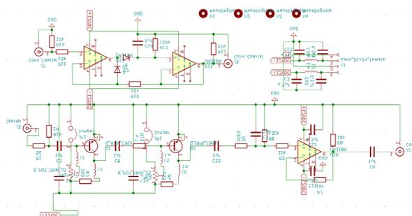
Figure 9: Schematics of active filter using BFU550 and signal buffer + peak detector (bottom).
