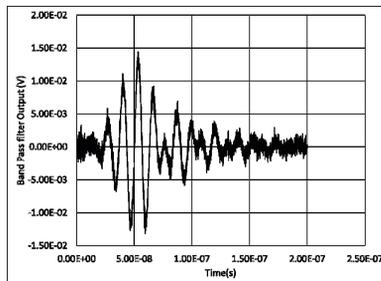
Figure 3: BPF (65 MHz to 85 MHz) output of button BPM signal from 30 nC electron bunch.
