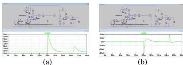
Figure 6: (a) Simulation with Class C + Class A amplifier; (b) simulation with Class A on both stages.
