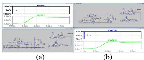
Figure 7: (a) Active filter using 2SC4083; (b) active filter using BFU550A. Both circuits have the same voltage buffer and peak detector.
