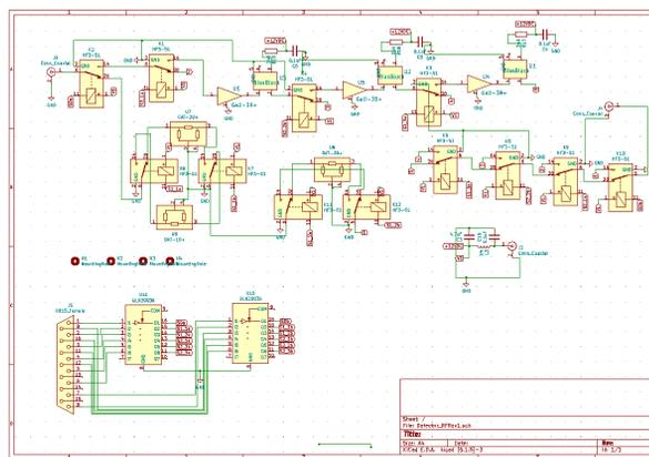
Figure 8: Schematics of RF switchyard.
