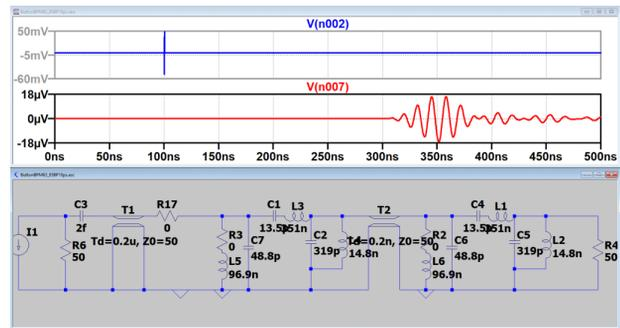
Figure 4: BPF simulation results of BPM signal.
