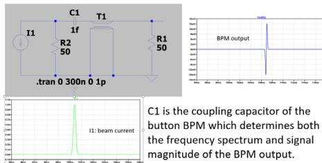
Figure 2: Equivalent circuit model of button BPM.
