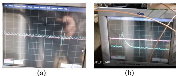
Figure 5: (a) Scope trace showing amplification of attenuated BPM signal; (b) scope trace showing active filter output and input signal.
