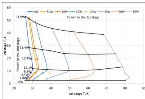
Figure 6: Cryocooler first and second stage temperatures at different input power levels to the stages.
