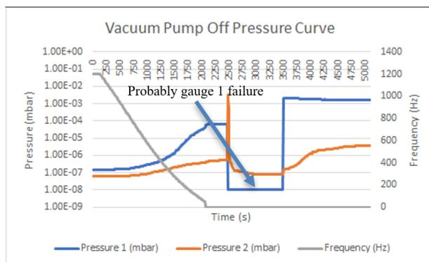
Figure 5: Pressure at the pump end (sensor 1) and the vacuum box (sensor 2).
