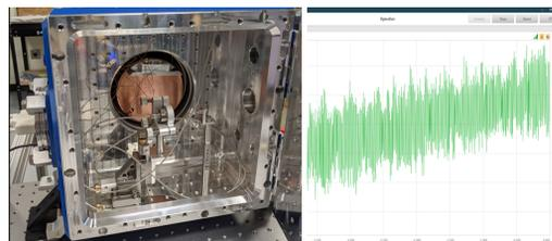
Figure 8: Vibration measurement setup in vacuum (left) and a 3.5 s sample (right).
