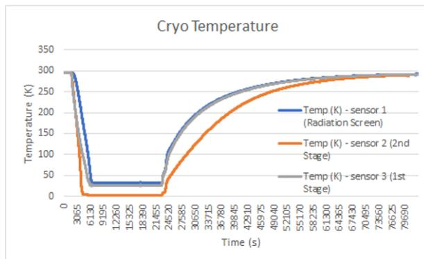
Figure 4: Temperature recorded during system cooldown and warm up with vacuum pump-off at 18000sec mark.
