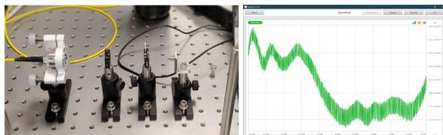
Figure 7: Vibration measurement setup in air (left) and a 5-s sample (right).
