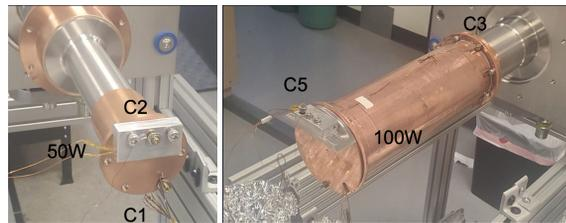
Figure 2: Temperature sensors: left – on the second stage cold head (C1) and heater block (C2); right – on the first stage (C3), at the end of the Cu radiation screen (C4, not seen) and the first stage radiation screen heater block (C5).
