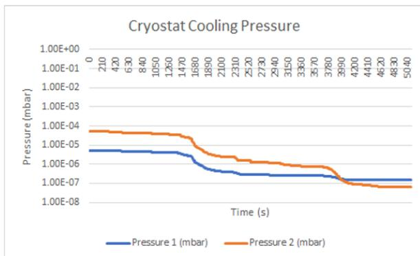
Figure 3: Pressure at the pump end (sensor 1) and the vacuum box (sensor 2).
