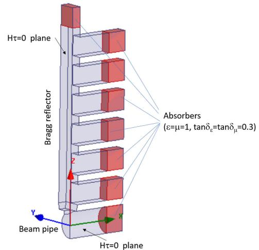
Figure 5: HFSS model for the open PBG resonator of QBPM.
