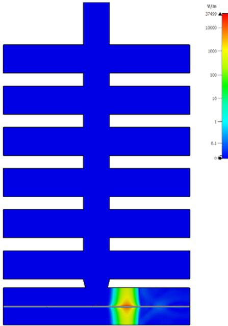
Figure 8: Instantaneous field when the bunch approaches to the resonator.
