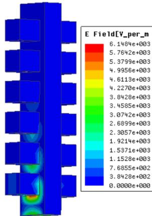
Figure 3: E-field structure of Bragg reflector at 10 GHz.
