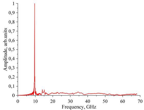
Figure 10: Fourier spectrum for the field excited in the PBG resonator.
