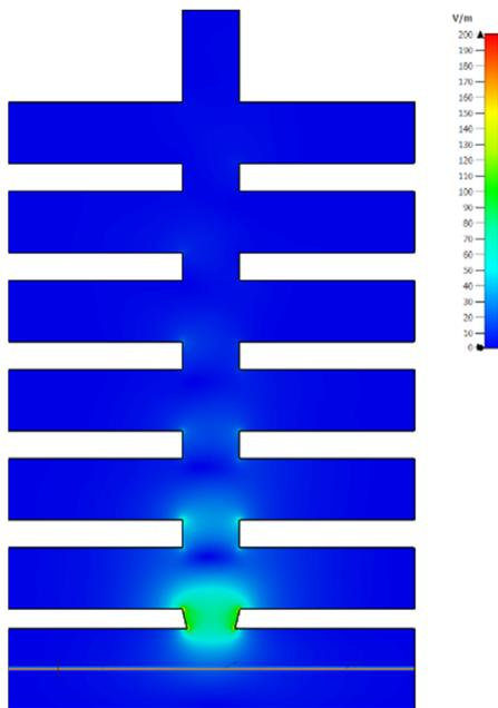
Figure 9: Instantaneous field distribution 10 ns after the bunch has passed.
