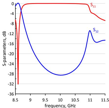
Figure 4: S-parameters of the reflector vs. frequency.
