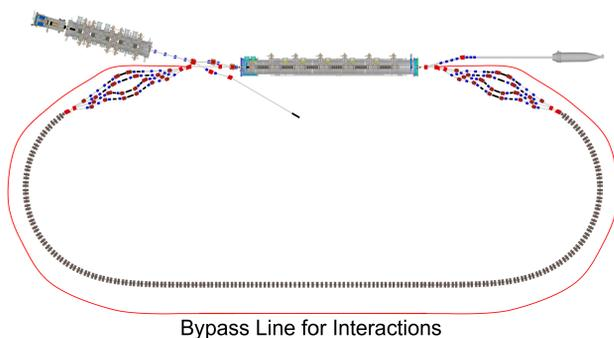
Figure 2: A cartoon layout of a multi-turn SRF ERL with an FFA arc and a bypass line for various applications, based on CBETA.
