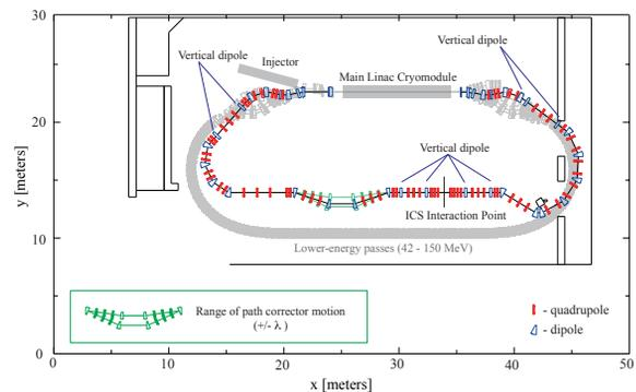
Figure 3: Layout of the ICS bypass in CBETA; grayed beam-line elements are already installed in the existing accelerator; originally published as Fig. 6 from [13].
