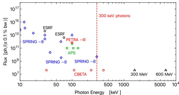
Figure 4: Flux per 0.1% bandwidth of the CBETA ICS (red) against a collection of the major high energy storage ring undulators across the globe; originally published as Fig. 12 from [13].
