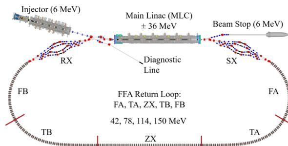
Figure 1: The four-turn configuration of CBETA.
