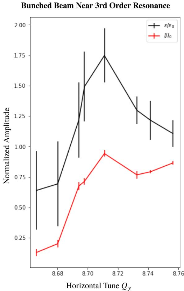
Figure 2: Saturated intensity and emittance of AGS experiments near resonance crossing. Growth seems consistent with that of high intensity bunched beam in SIS [1] including possible secondary resonance.
