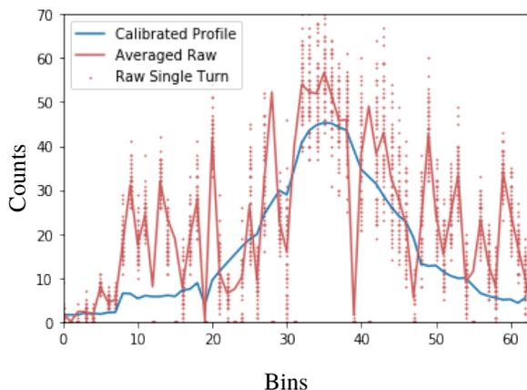
Figure 1: A vertical eIPM distribution taken at AGS injection. Raw profiles are in red, calibrated final profile is in blue. Any bins with obviously incorrect results are considered 'dead' and are removed from the data. Large tails are also observed, and are most likely overstated. Since this data is taken at injection, this is not due to the 3rd order resonance. Tails could be a calibration error or growth from the AGS Booster.
