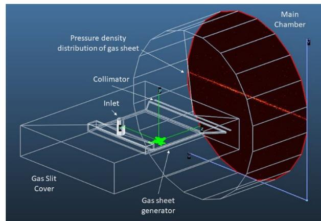
Figure 3: Molflow+ model showing the configuration of the simulation and distribution of the gas sheet at exit point.
