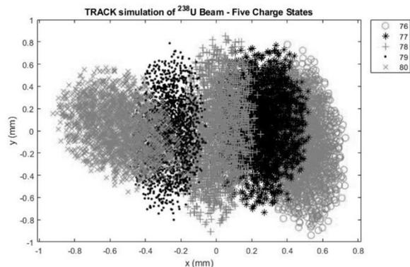
Figure 1: Example of charge state spread generated from TRACK simulation data at a 60 degree bend.
