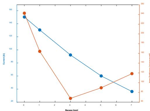
Figure 2: Extracted current and 4rms emittance at different cathode recess values.
