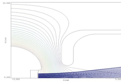
Figure 6: Design for a cathode with Pierce geometry.
