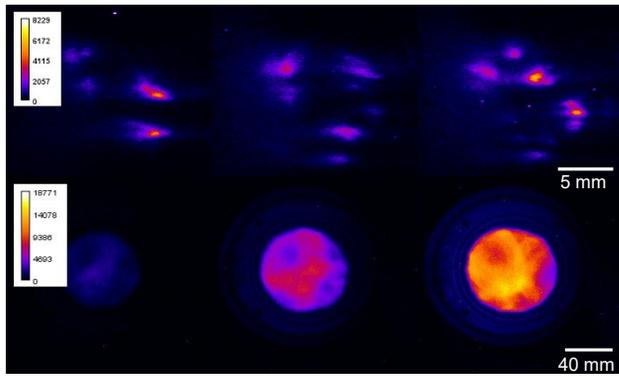
Figure 5: Images of the cathode (top) and scintillator (bottom) at differing diode voltages 269 ns into the pulse (left: shot 7086, middle: shot 7116, right: shot 7128).
