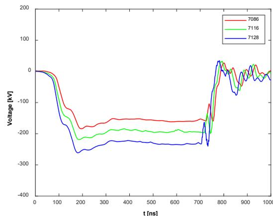
Figure 4: Diode voltage throughout a 700 ns pulse.
