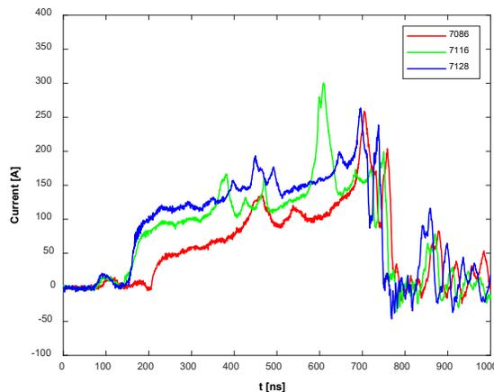
Figure 3: Extracted current throughout a 700 ns pulse.
