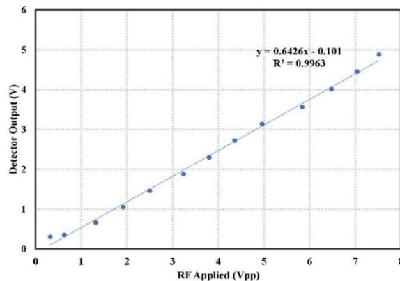
Figure 2: Linear fit of the peak-to-peak detector.
