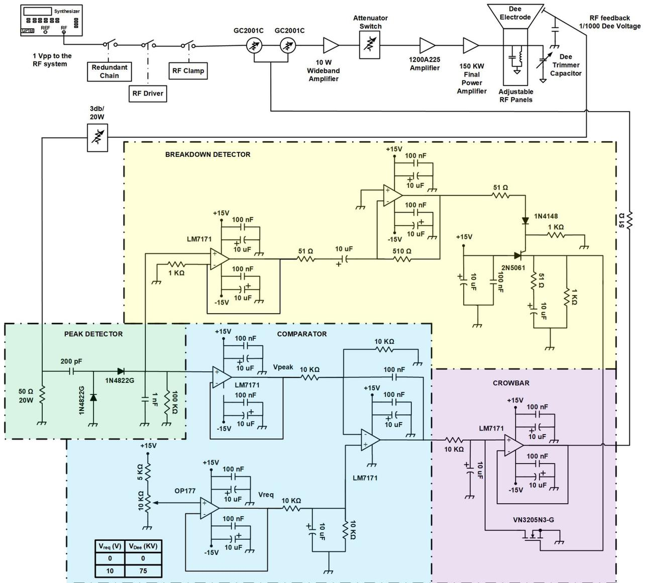
Figure 1: Dee voltage regulator interfaced with the RF system.
