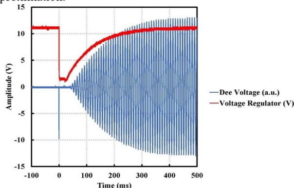
Figure 3: Recovery time of the Dee voltage after a RF sparking event is detected.
