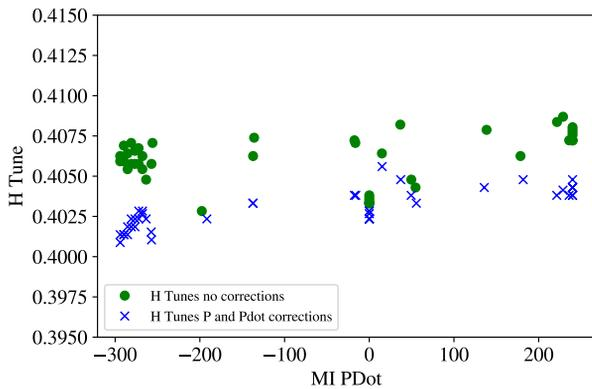
Figure 7: The horizontal and vertical tunes in the Recycler as measured at different points with respect to the MI ramp with  $P$  and  $\dot{P}$  corrections.
