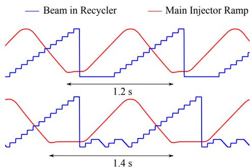
Figure 1: The position of the Recycler beam with respect to the MI ramp. When Muon campus is requesting beam, the MI ramp sits at 8 GeV for extra 0.2 s.
