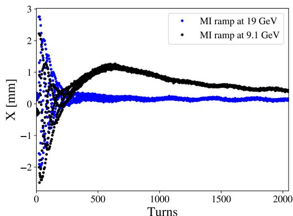
Figure 3: Example tbt data showing the effect of the MI ramp on the horizontal beam position at two different momentum during the MI ramp. The initial amplitude increase is from the ping for tune measurements.
