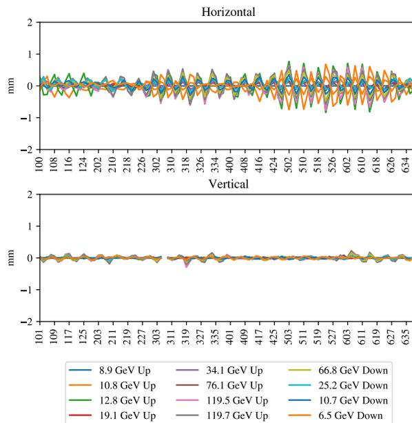
Figure 5: Recycler difference orbits taken at various MI ramp momentum breakpoints with MI ramp compensation enabled.
