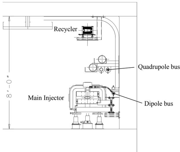
Figure 2: A schematic of the Main Injector enclosure which holds both the Main Injector and Recycler accelerators.
