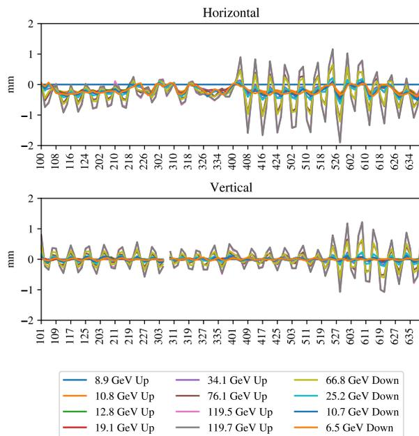
Figure 4: Recycler difference orbits taken at various MI ramp momentum breakpoints with no MI ramp compensation enabled.
