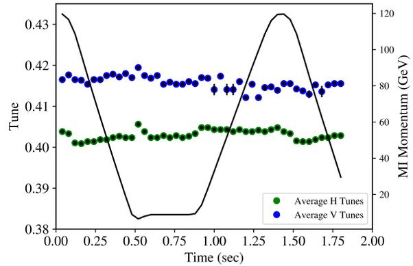
Figure 8: The horizontal and vertical tunes in the Recycler as measured at different points with respect to the MI ramp with  $P$  and  $\dot{P}$  corrections.
