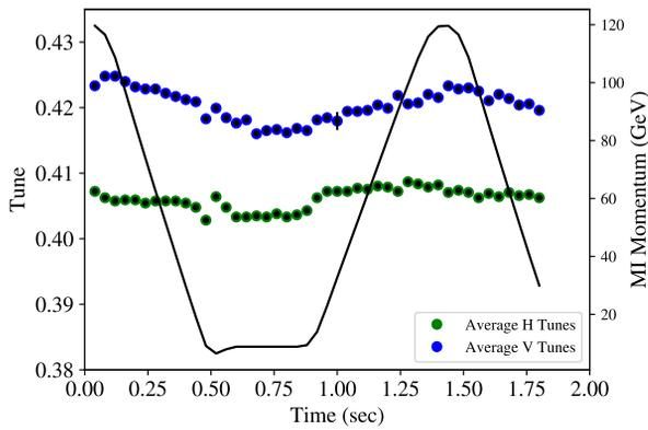
Figure 6: The horizontal and vertical tunes in the Recycler as measured at different points with respect to the MI ramp.
