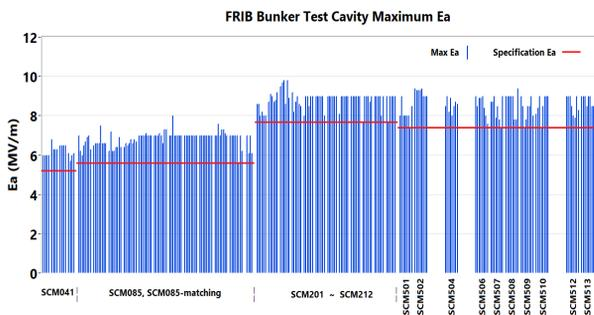
Figure 3: Gradients reached in bunker tests. Blue bar: measured gradient; red line: FRIB requirement.
