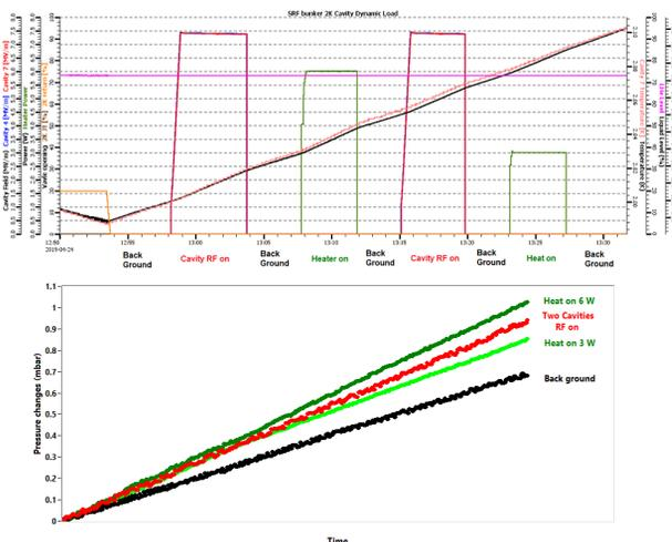
Figure 6: Dynamic heat load measurement at 2 K. Top: bath pressure (black), cavity fields (blue, red), and heater power (green) as a function of time. Bottom: zoomed-in  $P$  as a function of  $t$  (red: both cavities on; dark and light green: heater on; black: cavities and heater off).
