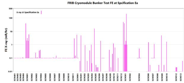
Figure 4: Field emission X-rays measured at the operational gradient in bunker tests.
