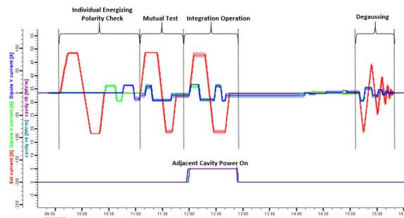
Figure 8: A typical solenoid package bunker test. Red: solenoid current; green: dipole  $x$  current; blue: dipole  $y$  current (from Ref. [4]).
