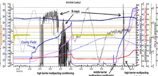
Figure 2: Conditioning of multipacting for a  $\beta = 0.53$  HWR (SCM508, Cavity 2): cavity field (blue), X-rays (black), forward power (pink), and coupler temperature (red).
