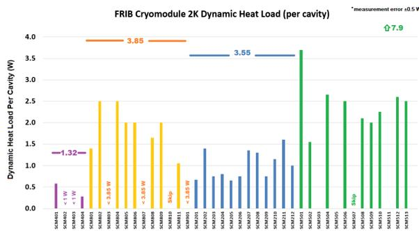
Figure 7: Estimated dynamic heat load per cavity at 2 K.
