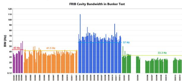
Figure 1: Measured cavity bandwidths.
