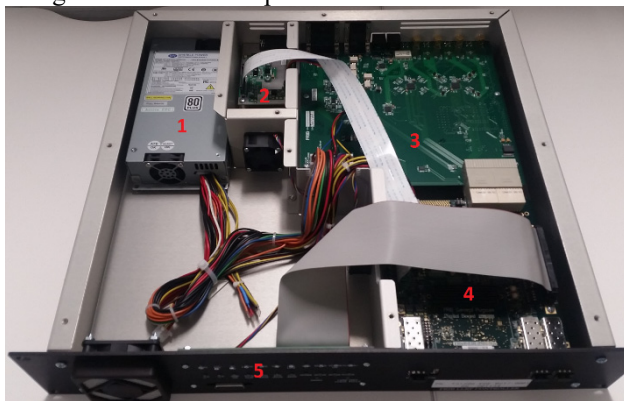
Figure 2: FRIB LLRF controller. 1. Power supply; 2. Tuner board; 3. RF board; 4. FGPDB; 5. Front panel and board.
