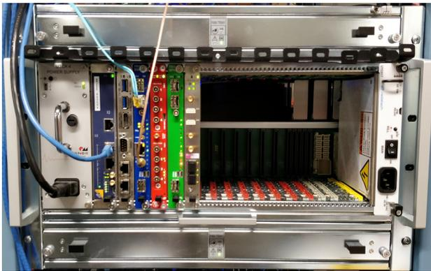
Figure 1: A  $\mu$ TCA crate with MCH, CPU, Event Receiver, Pico8, BPM and BCM cards.
