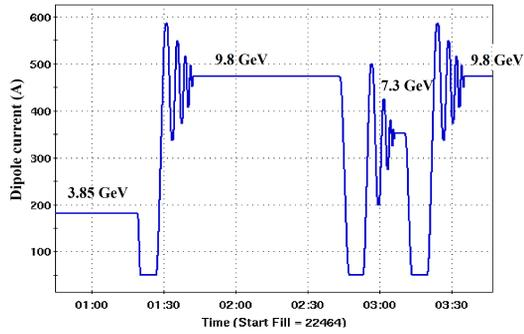
Figure 1: The dipole current was switched from that for 3.85 GeV/nucleon to 9.8 GeV/nucleon, to 7.3 GeV/nucleon and back to 9.8 GeV/nucleon. System settings are automatically restored for the various energies during the switches. One demagnetization cycle was exercised on the dipole magnet to stabilize the field for beam operation.
