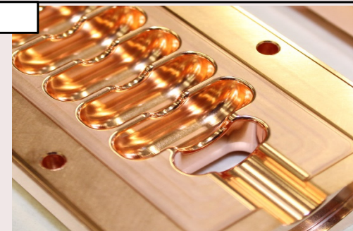
Novel split-block assembly for novel gap accelerator
