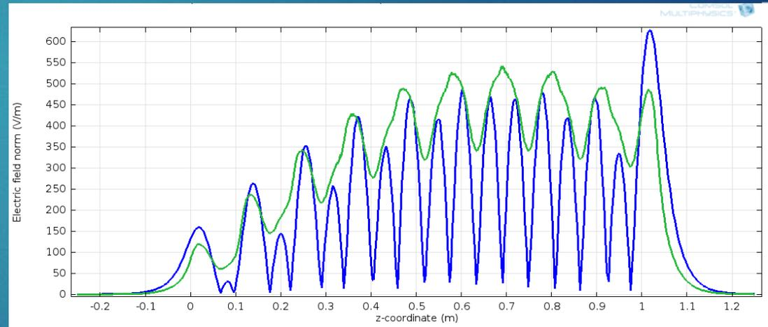
Higher harmonics can potentially move the peaks in the electric field from the equator to near the irises of the cavity.
