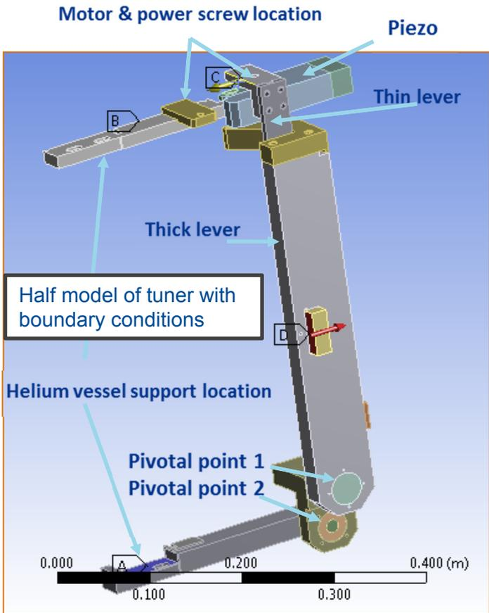
Half model of tuner with boundary conditions
