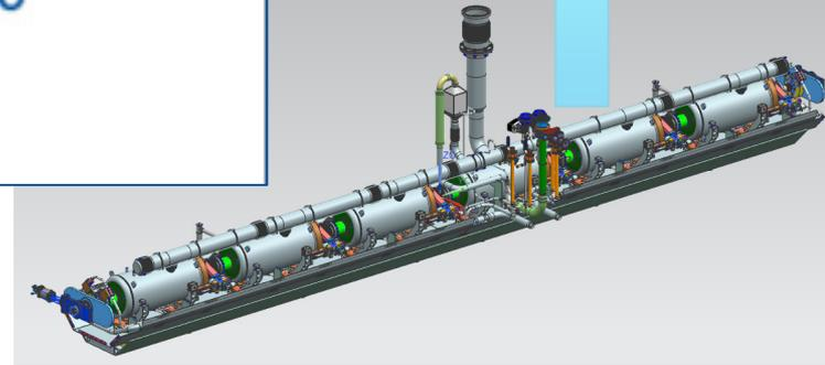
**Different BC as compared to ILC cavity due to Bottom supported cavity in CM**
