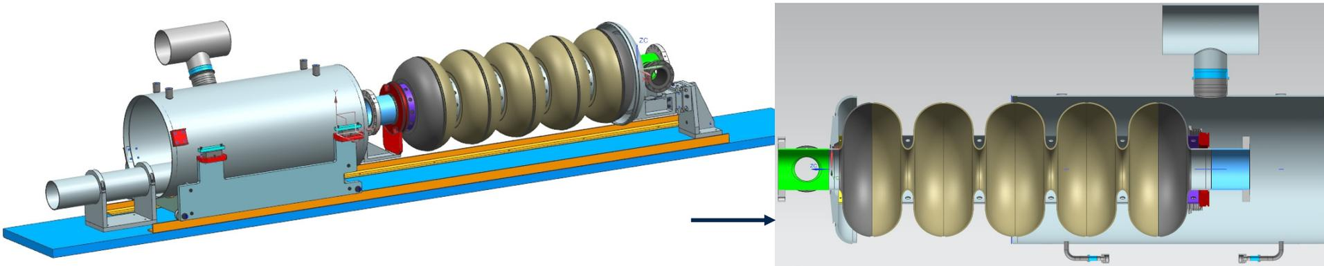
Insertion device (medium bertha) for cavity dressing
