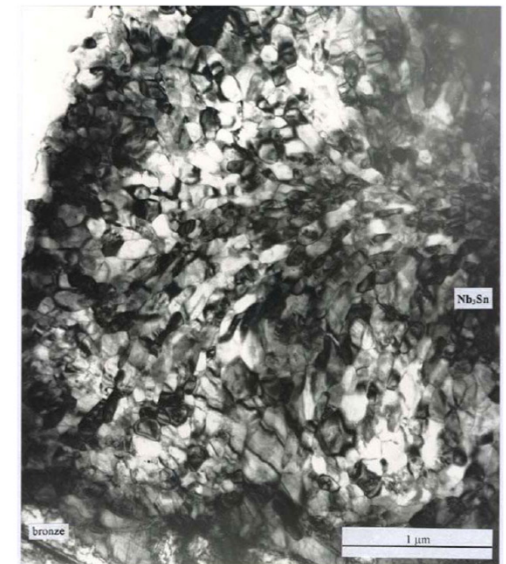
Fig. 6: Microstructure of a Nb 3 Sn filament (Courtesy of C. Verwaerde, Alstom/MSA).
