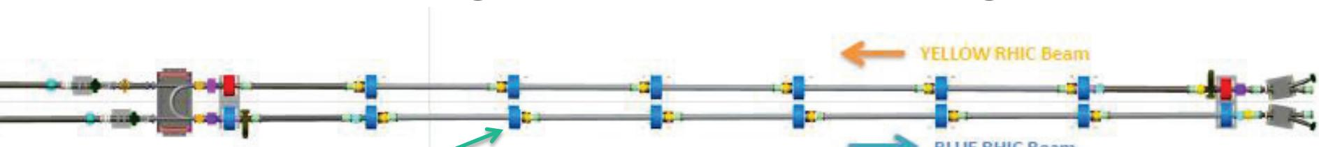
Distance covered by magnetic field from solenoids will be lost from cooling. Expect about 40 cm to be lost from cooling from each solenoid.
