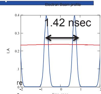
9 MHz RHIC RF LReC Beam Structure
