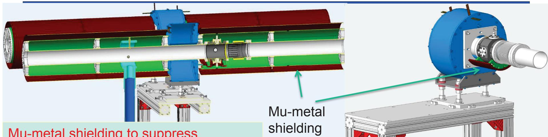
Mu-metal shielding to suppress transverse magnetic fields to required level in free space between the solenoids (cooling region).
