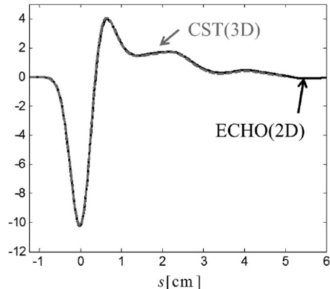
Longitudinal wake potential of tapered collimator
