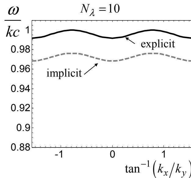
No dispersion in z-direction + no dispersion along XY diagonals
