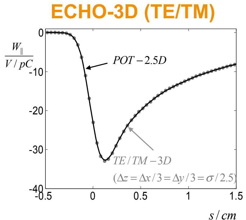
Comparison of the wake potentials obtained by different methods for structure consisting of 20 TESLA cells excited by Gaussian bunch  $\sigma = 1mm$
