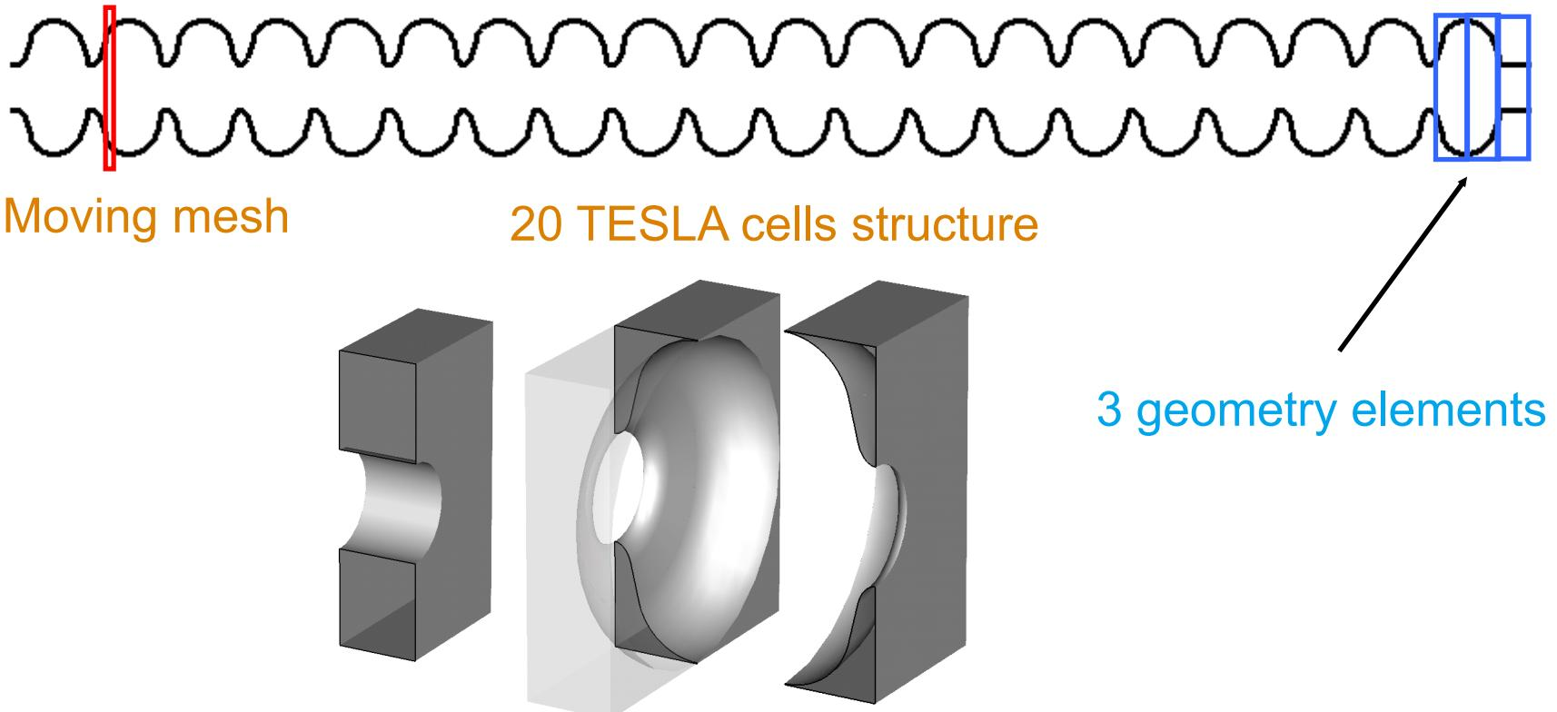
The geometric elements are loaded when the moving mesh reaches them. During the calculation only 2 geometric elements are in memory.
