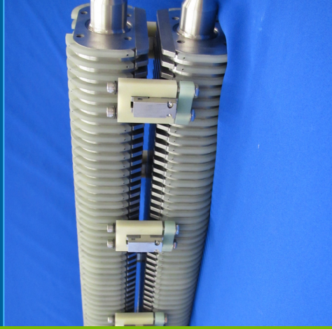
Assembled cores before winding and epoxy impregnation
