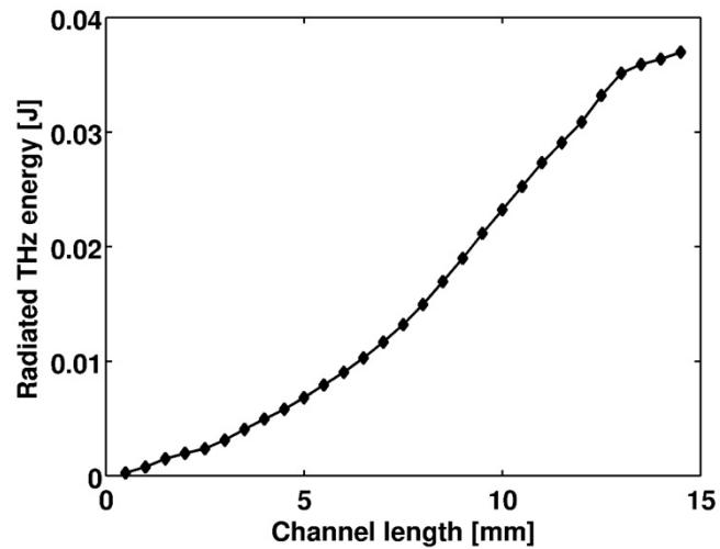
THz energy of 38 mJ is generated, more than 8% of the depleted pulse energy is converted into THz radiation.
