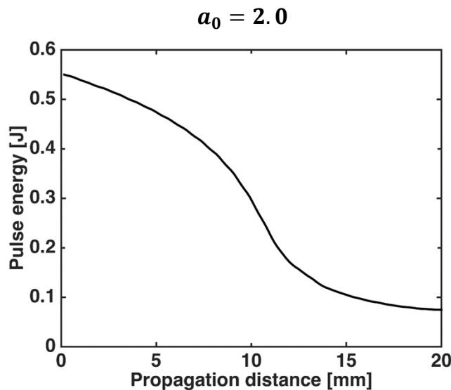
Around 80% of the energy stored in the laser pulse is depleted within the propagation distance of 1.5 cm\*
