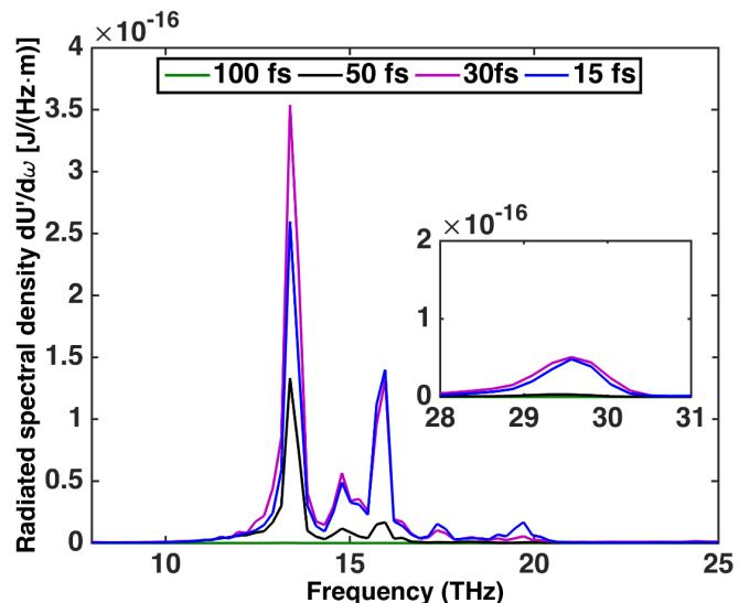
The fundamental mode is enhanced using a optimum pulse duration of 30 fs.
