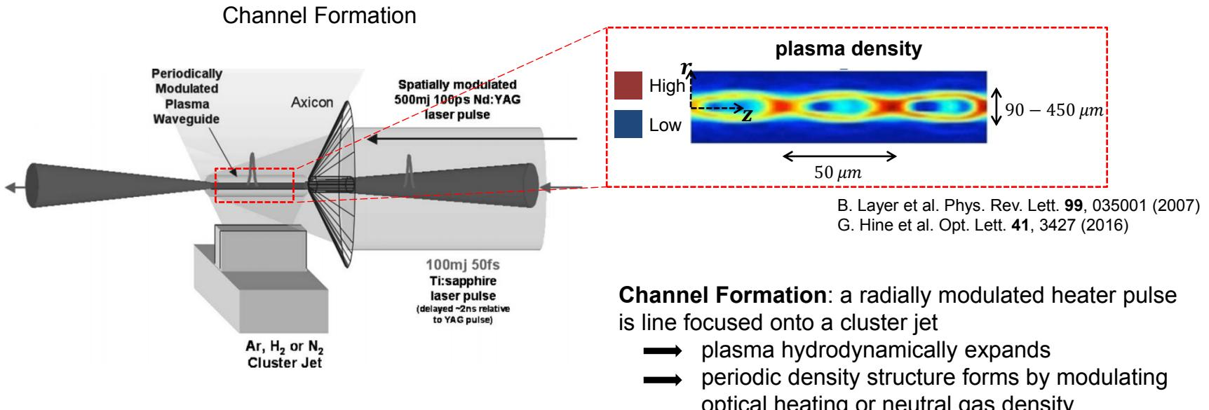
**Channel Formation:** a radially modulated heater pulse is line focused onto a cluster jet
