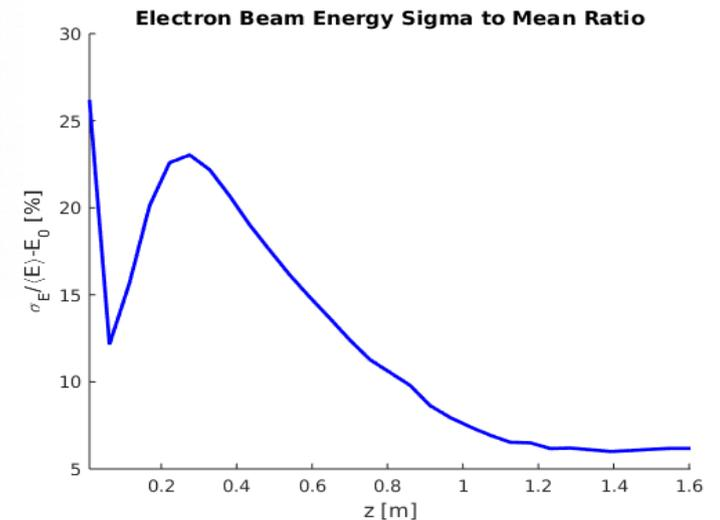
Here we achieved a good balance between energy spread and the amount of charge accelerated. But: initial charge was 201 pC, and has dropped to 153 pC.
