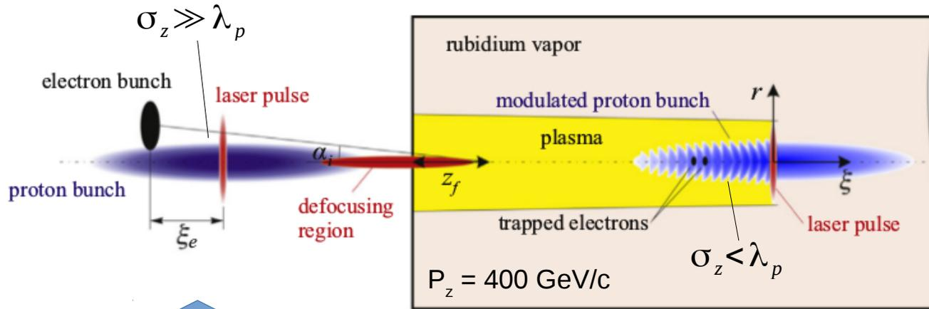
The oblique injection of the electrons into the plasma.
