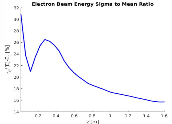
Initial charge was 401 pC in this case. Energy spread is increasing as the beam gains energy.
