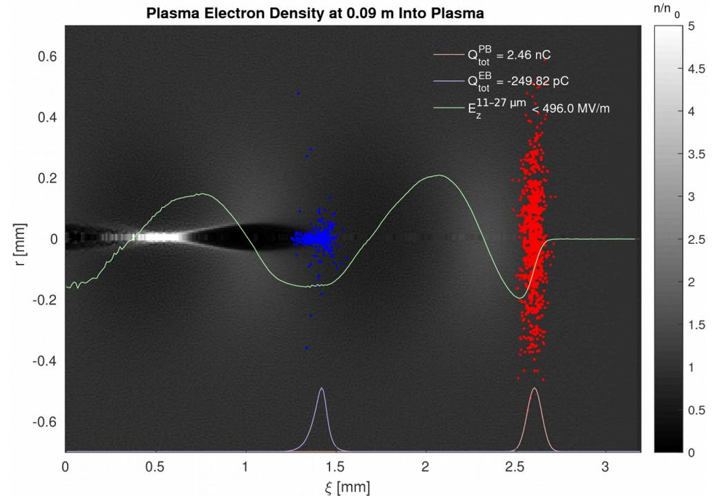
A single, 2.5 nC, proton driver with a 250 pC electron witness beam. The minimum plasma electron density in the bubble created by the driver is  $\sim 0.6$ .
