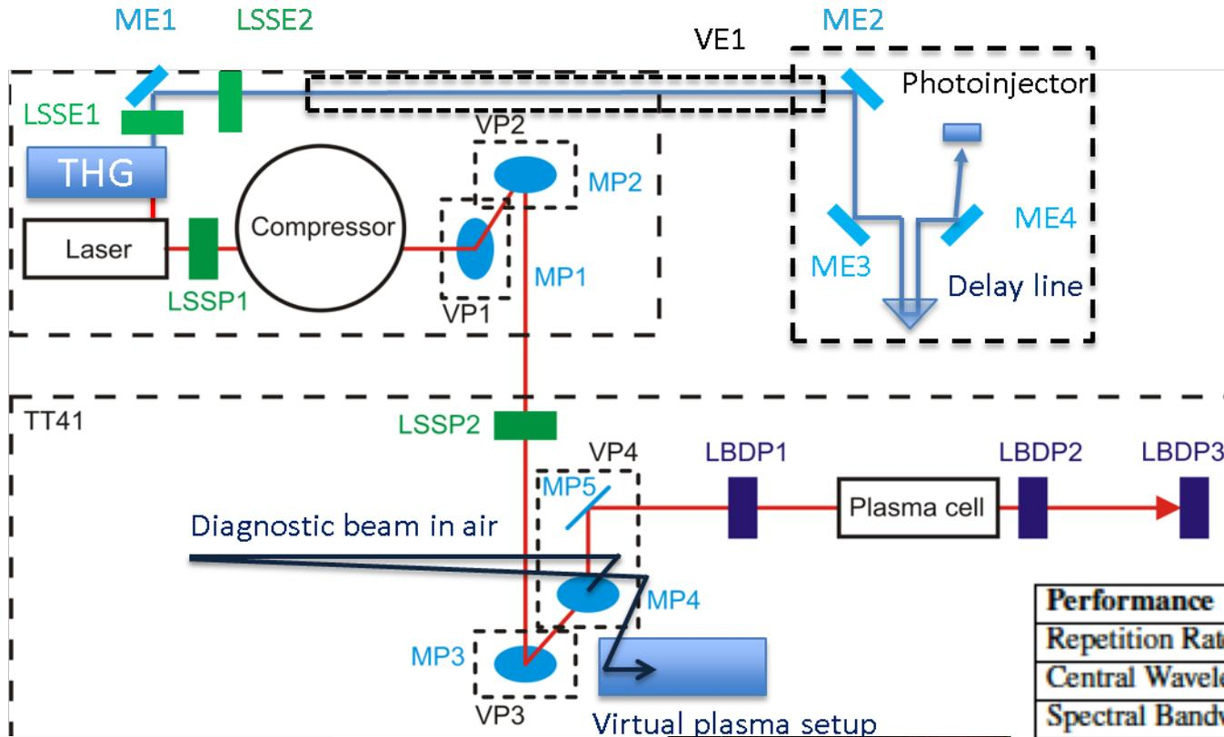
Laser beam setup – includes a ‘virtual plasma cell’ line for commissioning & monitoring laser.
