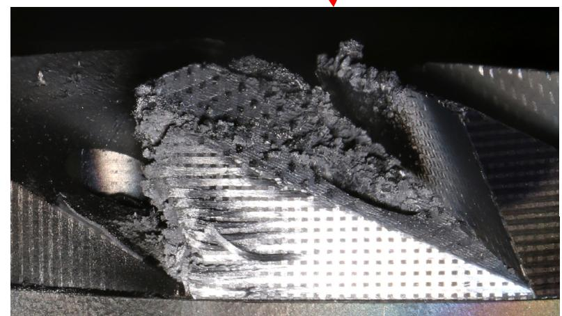
Electron collector damage
