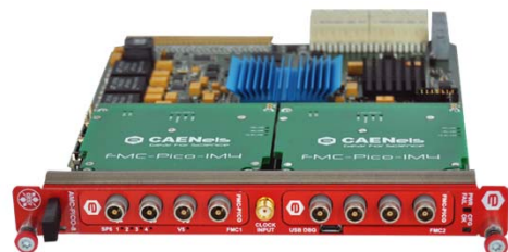
CAENs AMC-PICO-8 8 chan @ 1MS (35kHz BW ) 65x Halo Ring Monitors 42x Ion Chambers 24x Neutron Detectors
