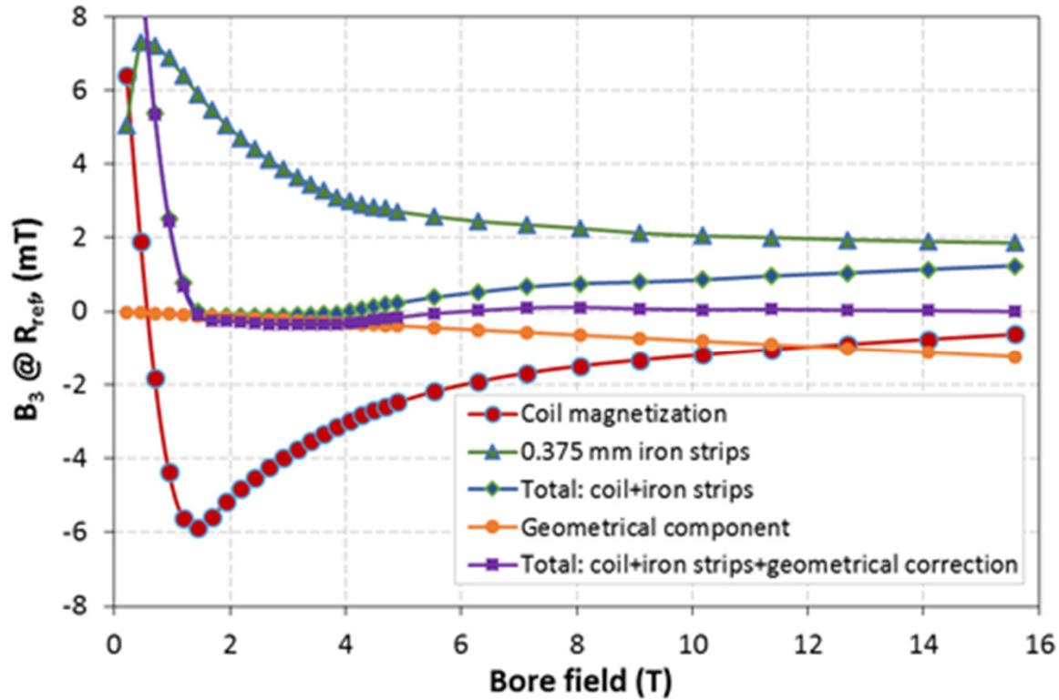
0.375 mm iron strips in aperture at 50-75 degrees in each quadrant and geometrical component  $b_3 = -0.8$  units.
