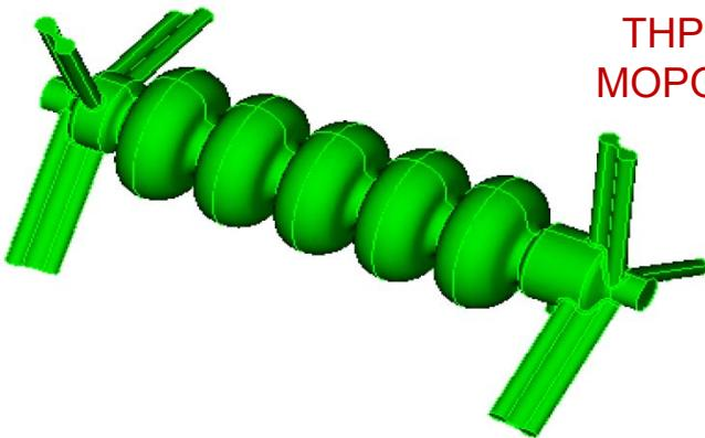
650 MHz cavity with ridge waveguide dampers
