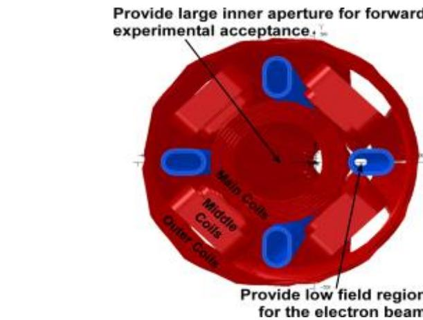
ERL-ring design: “Sweet spot” IR magnet design concept arranges a field-free electron pass between SC coils.
