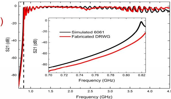
Ridge WG is a natural high pass filter with higher bandwidth, smaller size than regular WG.
