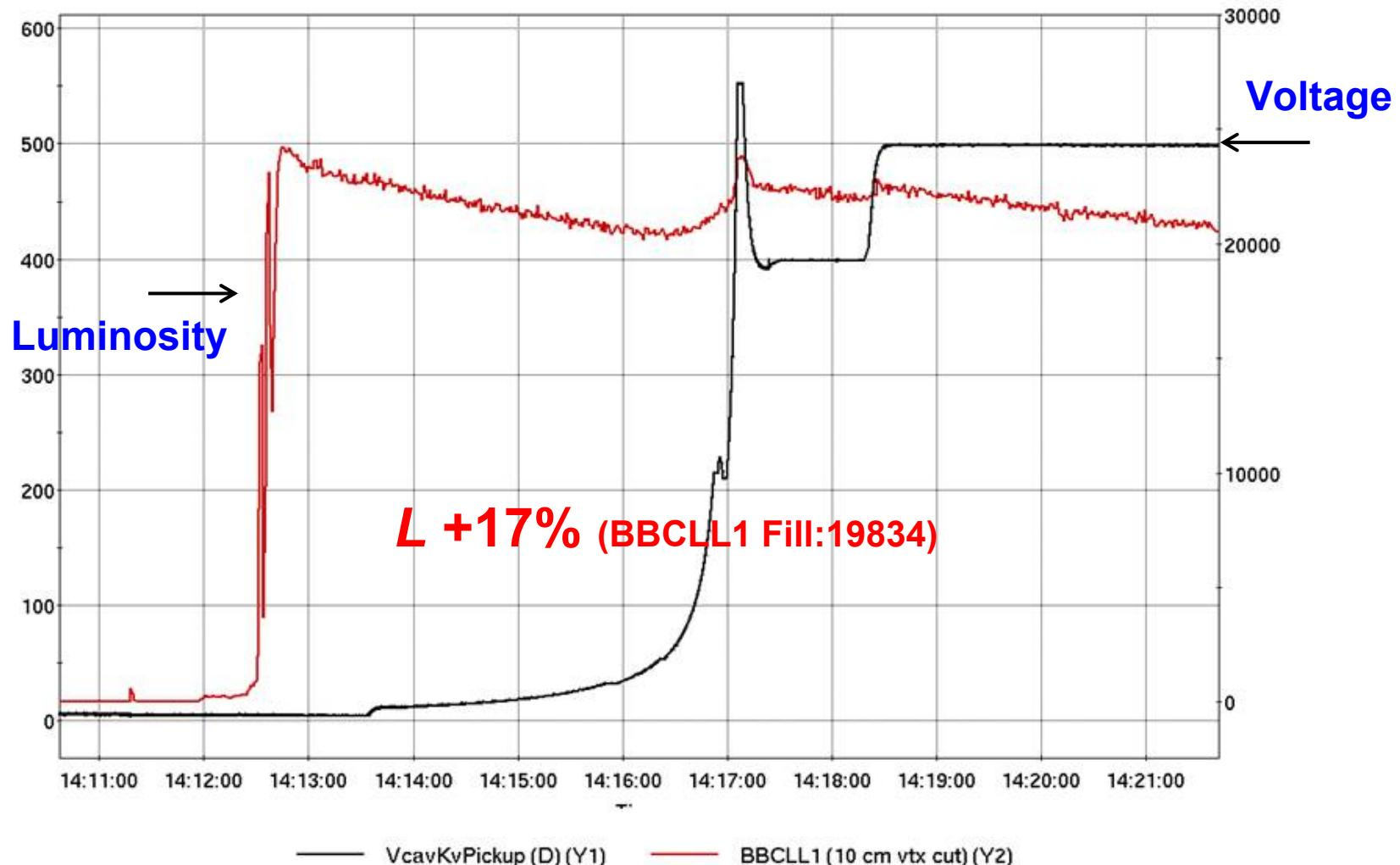
Has achieved 1 MV cavity voltage during 100 GeV Au-Au run without HOM damper.
