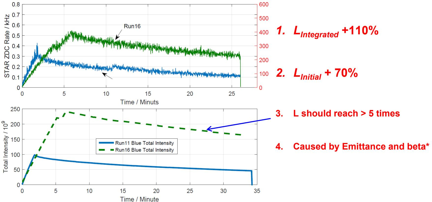
1. Run16 Integrated STAR luminosity is **2.1** times of Run11 and 1.7 times for initial luminosity.
