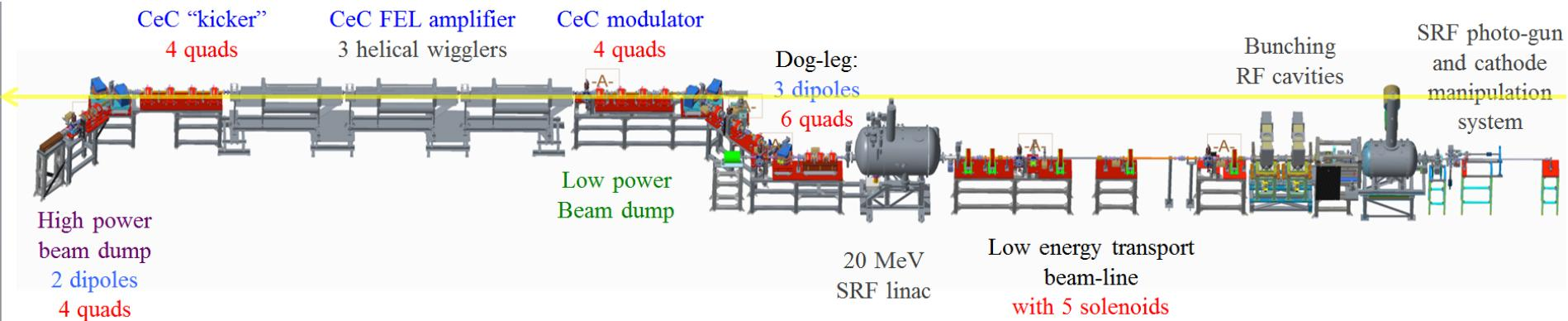
1. Coherent electron Cooling is a novel cooling technique for potential application in eRHIC.
