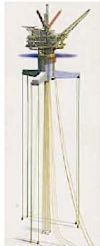
Tension Leg Platform
