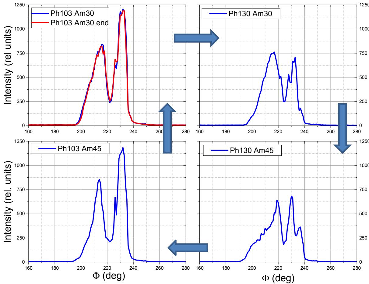
$H^+$  ion bunch shape changes on variations of prebuncher phase and amplitude.
