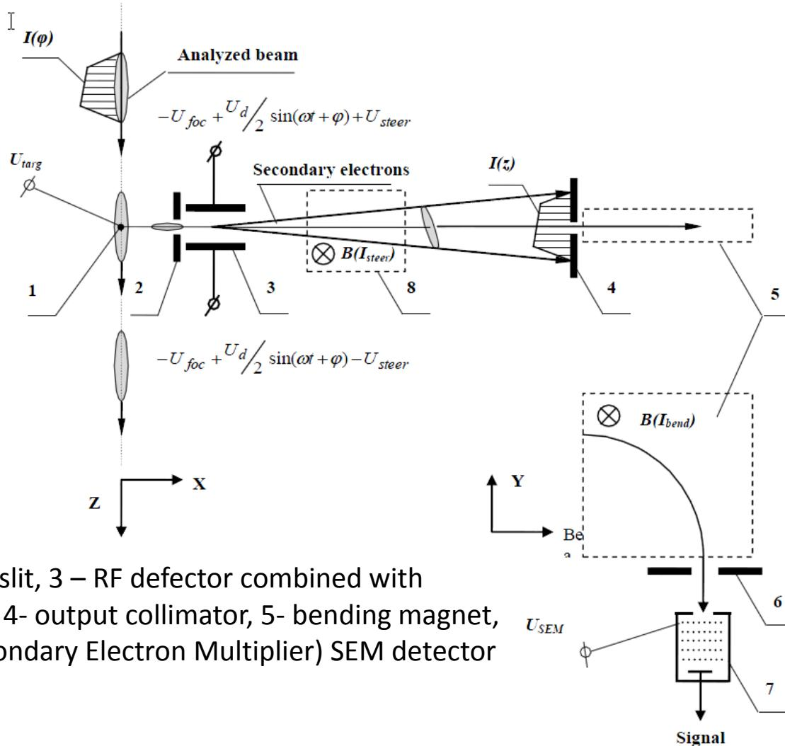
1-Target, 2- input slit, 3 – RF defector combined with electrostatic lens, 4- output collimator, 5- bending magnet, 6-collimator, (Secondary Electron Multiplier) SEM detector
