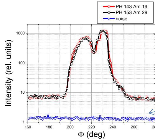
$H^+$  ion bunch shape changes on variations of prebuncher phase and amplitude.
