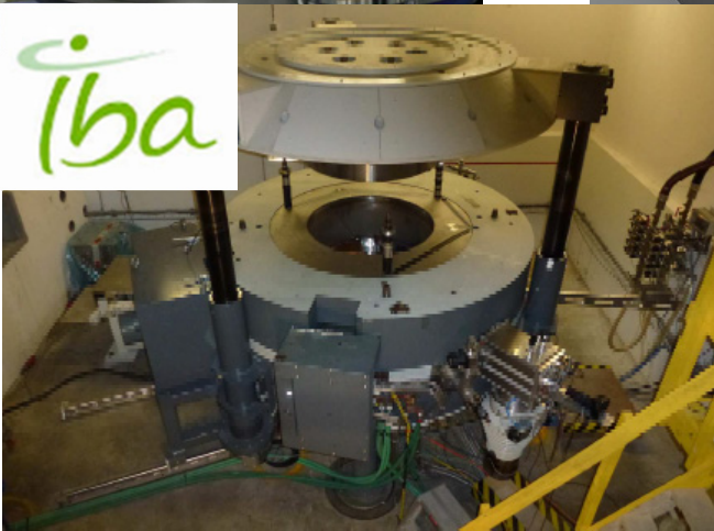
SC Cyclotrons used by IBA and Varian
