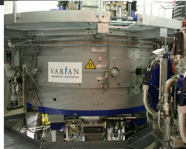
SC Cyclotrons used by IBA and Varian
