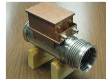
Short version of the Switchyard Resonant BPM, tuned to 53.10348 MHz using a coil inductor
