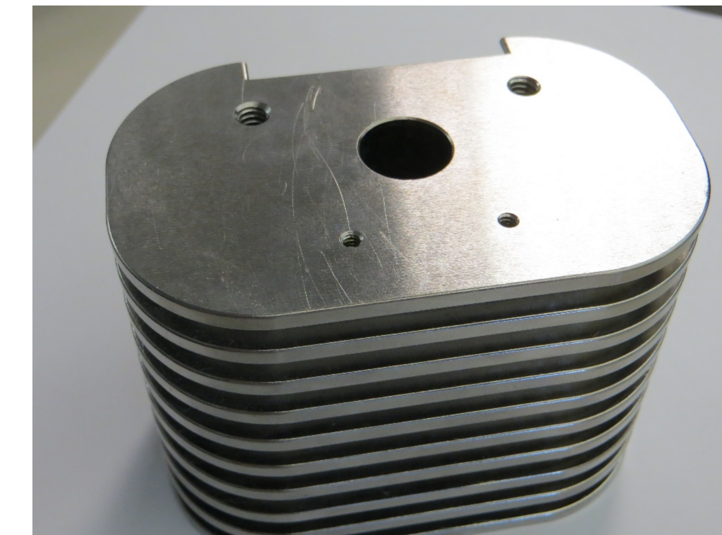
First Design of the Magnet Structure Jaw for the Planar Superconducting Undulator
