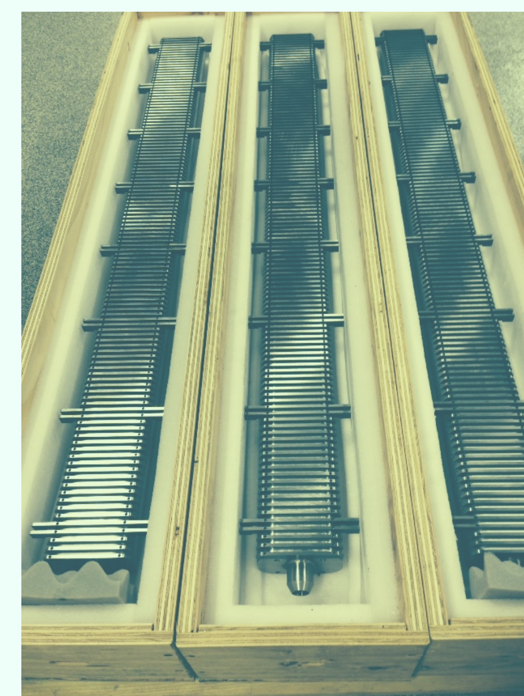
1.5-meter-long magnet structures precisely machined according this technology
