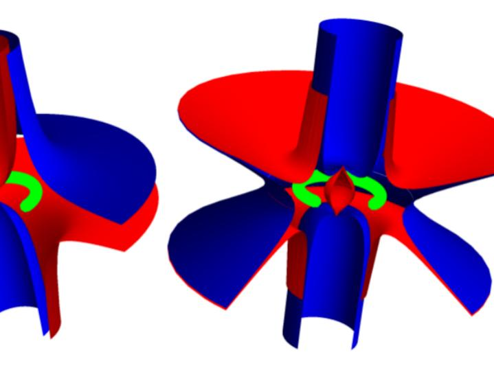
3D models of 2n-pole sector magnets. From the left to the right: skew S-dipole, normal S-dipole, skew S-quadrupole, normal S-quadrupole and skew S-sextupole.
