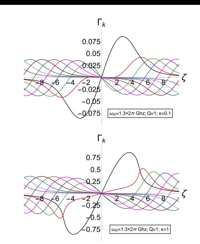
Left figure shows another example: single Gaussian bunch in FNAL Recycler (resistive wall wake). Now the only growth rate of the most unstable mode as a function of the head-tail phase and gain of resistive damper is plotted. As has been expected for  $0 < \zeta < 1$  and  $g \sim 1$  there is a "Lake of Stability" where all modes have negative growth rates [4].
