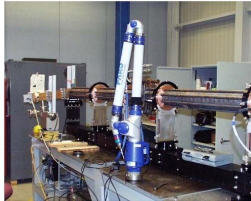
Figure 5: Linac structure on strong-back with supports and portable CMM.
