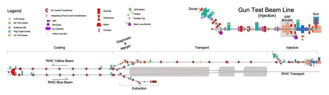
Figure 1: Layout of LEReC electron accelerator showing the five sections. An enlarged view of the injection section as it will be set up during the Gun Test is shown on the right.
