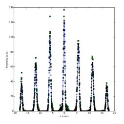
Figure 2: The horizontal projection of the beam stripes on the profile monitor for beam energy of 0.4 MeV, and the multiple Gaussian peak fitting of the projection.
