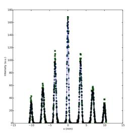
Figure 4: The horizontal projection of the beam stripes on the profile monitor for beam energy of 2.6 MeV, and the multiple Gaussian peak fitting of the projection.
