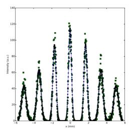
Figure 3: The horizontal projection of the beam stripes on the profile monitor for beam energy of 1.6 MeV, and the multiple Gaussian peak fitting of the projection.
