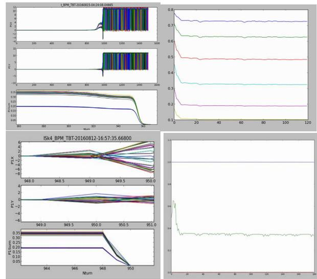
Figure 4: beam loss localization from AI and kicker trip.
