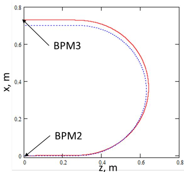
Figure 5: 5% off energy beam trajectory (solid red line) and reference on-energy beam trajectory (dotted blue line) in the realistic soft-edge dipole. The simulations of the off-energy beam trajectory include all the errors listed above.
