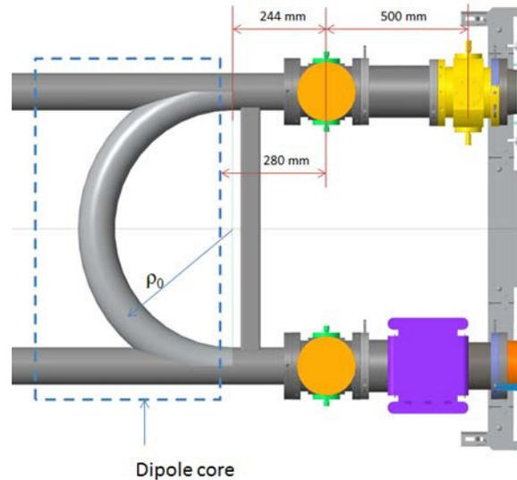
Figure 2: Schematics of  $180^\circ$  bend.
