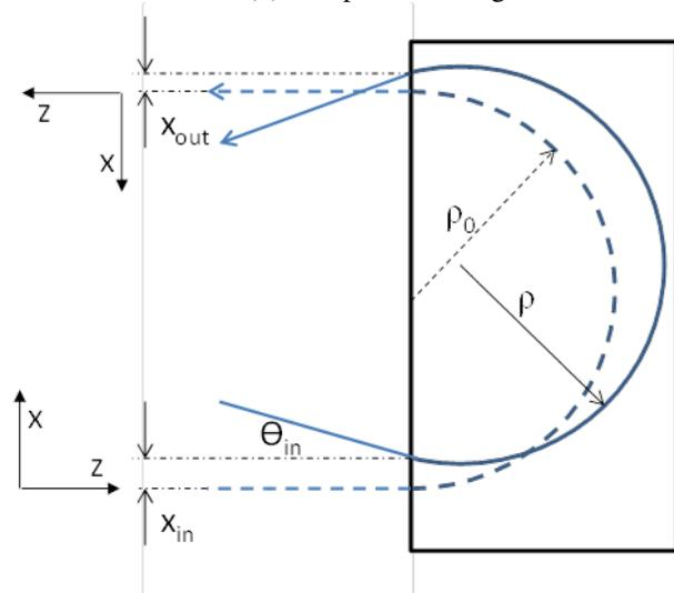
Figure 3: Beam trajectory in  $180^\circ$  bend.
