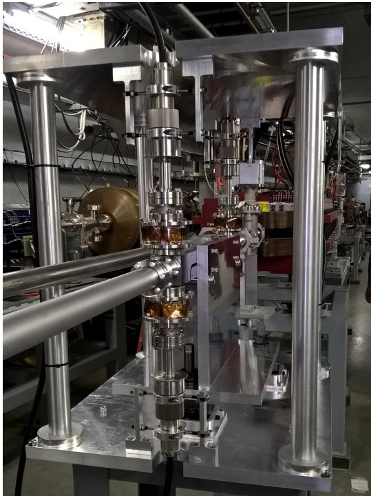
Figure 5: The kicker installed in the BTX beamline.
