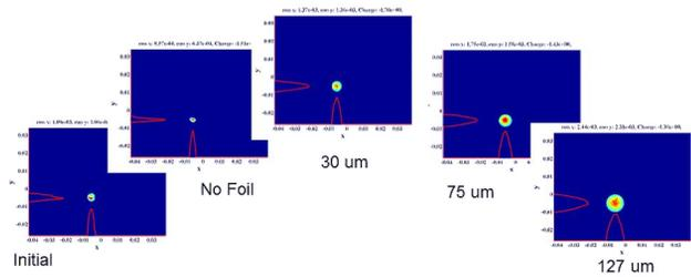
Figure 2: A representative example of the 45 MeV intensity distributions with the projections from fits for the initial spot at YAG1 and the spots at YAG2 for case of each Be foil and no foil.
