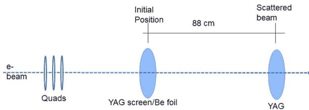
Figure 1: Schematic of the experimental setup. The electron beam propagated from the left, charge measured with an ICT (not pictured) before the foil. The beam was focused by 3 quadrupoles. The image was recorded at the two YAG screens located 88 cm apart, YAG1 at the Be foil position and YAG2 88 cm downstream.
