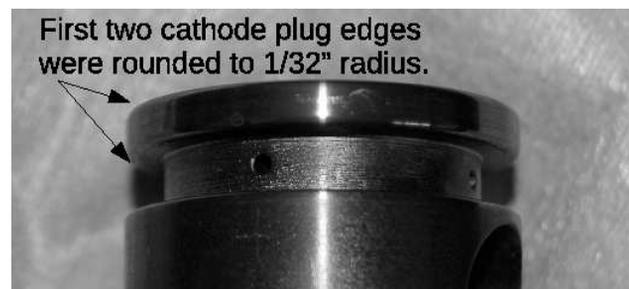
Figure 3: The rounded edges (radius 1/32 in.) eliminated the arcing in the gap.
