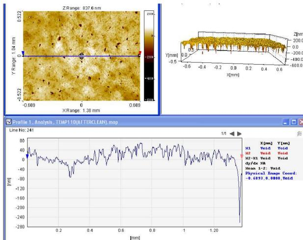
Figure 5: Cathode1 plug surface analyzed in the white light interferometer, after cleaning. Features are now on the order of 100s nm in scale. This suggests that the spots are places that the cathode film was damaged, in some cases removed down to the Mo surface.
