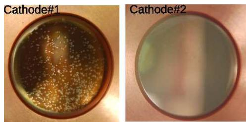
Figure 2: Pictures of Cathode1 (left) and Cathode2 (right) in the gun. On Cathode1, an estimated 600 spots developed, mostly during the month-long RF conditioning to 88 MV/m. Despite the appearance of the spots during RF conditioning, the photocathode performed fairly well for nearly 2 years of operation. However, the cathode started arcing uncontrollably and had to be replaced. Cathode2 is the replacement and has operated for 1 year with high QE, fast conditioning, and no arcing problem.
