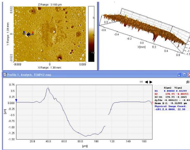
Figure 4: Cathode1 plug surface analyzed in the white light interferometer, before wiping off the surface. Micron scale pits and features.
