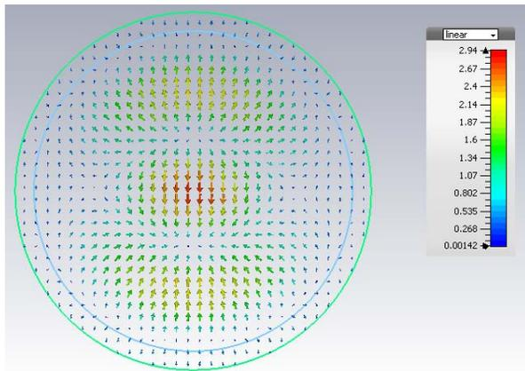
Figure 2: H field plot for HEM<sub>12</sub> mode in amps/m.
