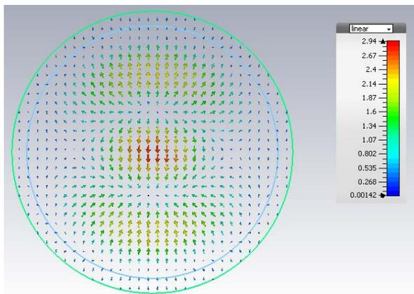
Figure 2: H field plot for  $HEM_{12}$  mode in amps/m.
