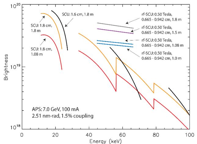
Figure 3: X-ray brightness, ph/s/mrad<sup>2</sup>/mm<sup>2</sup>/0.1%bw, as a function of x-ray energy for the  $HEM_{12}$  example WG over the frequency range of 18-GHz to 24.5 GHz and for various lengths. Comparison plots are also made for the existing APS SWU (1.8cm, 1.08 m) and possible future SWUs.
