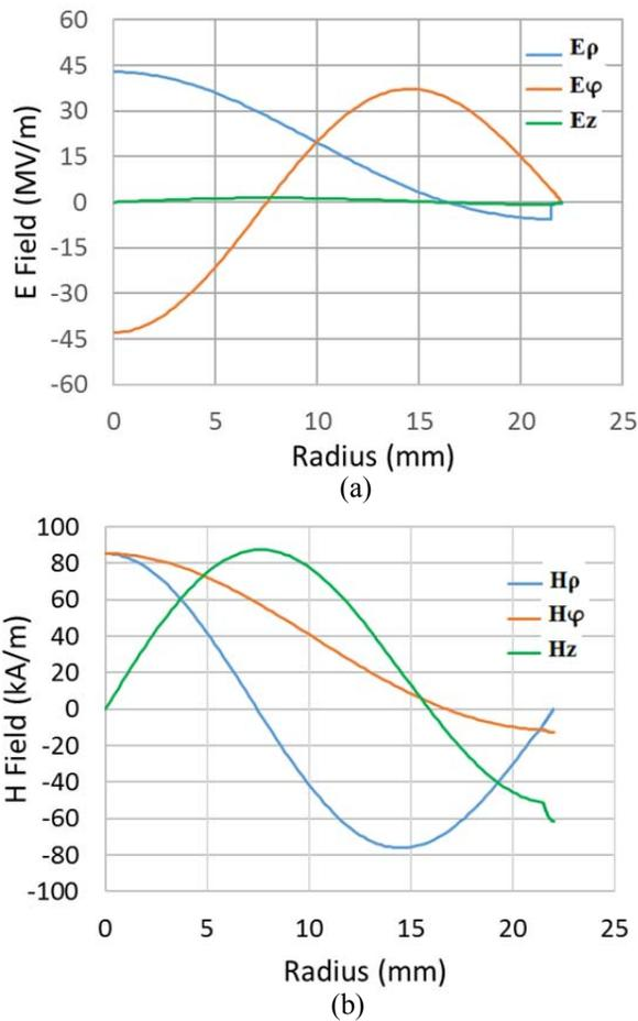
Figure 1: Field components for a  $HEM_{12}$  mode along radial direction: (a) Electric Field and (b) Magnetic intensity.
