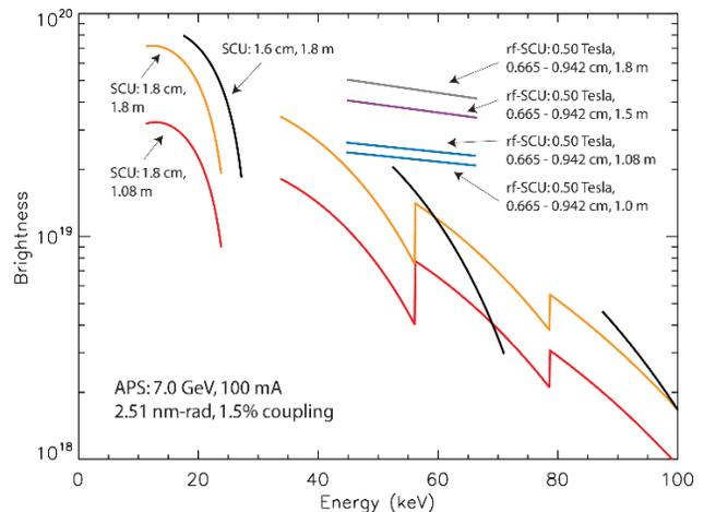
Figure 3: X-ray brightness, ph/s/mrad<sup>2</sup>/mm<sup>2</sup>/0.1%bw, as a function of x-ray energy for the HEM<sub>12</sub> example WG over the frequency range of 18-GHz to 24.5 GHz and for various lengths. Comparison plots are also made for the existing APS SWU (1.8cm, 1.08 m) and possible future SWUs.
