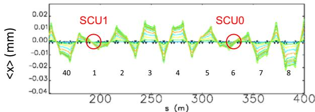
delay, it was confirmed that the SCUs did not quench when energized to typical operating values. A kicker setpoint of 8 kV showed somewhat higher BLM losses, even though simulations showed no losses. In all cases, the losses at ID6 are  $< 1$  nC, which is consistent with quench prevention [1,2]. Unlike ID1, the ID6 SCU photon absorber does not intercept aborted-beam losses, and the abort system protects ID6 SCU with or without the delay.
