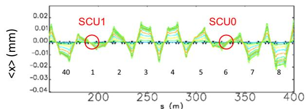
Figure 3: Simulated beam trajectories for 24 bunches and kicker voltage setpoint of 8 kV (1.0 mrad peak kick), showing about one third of the first turn after the kick. The abort kicker is located in S36 and the target loss location is S39. The sector straight sections are labelled.
