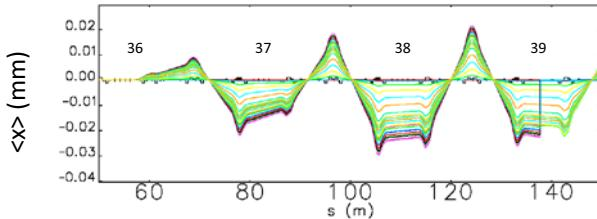
Figure 3: Simulated beam trajectories for 24 bunches and kicker voltage setpoint of 8 kV (1.0 mrad peak kick), showing about one third of the first turn after the kick. The abort kicker is located in S36 and the target loss location is S39. The sector straight sections are labelled.
