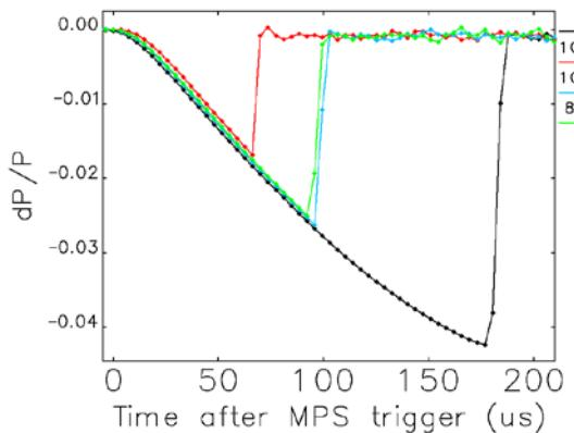
Figure 5: Beam energy as a function of time after MPS trigger event. The moment of beam loss corresponds to the energy reverting to zero.
