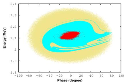
Figure 3: Longitudinal acceptance of the PIP-II SC linac (cyan) with  $6\sigma$  beam at upstream of the linac (red). Initial particle distribution is shown in khakee.
