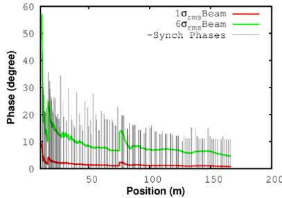
Figure 2: Accelerating phases in cavities for nominal configuration of the PIP-II SC linac.
