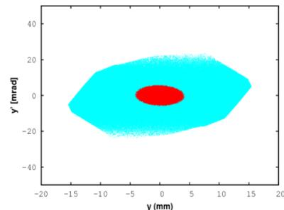
Figure 5: Transverse acceptance of the PIP-II SC linac (cyan) with  $6\sigma$  beam at upstream of the linac (red).
