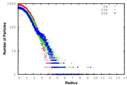
Figure 6: Longitudinal particle distribution at the end of PIP-II SC linac. (Radius =  $|\sigma|$ )
