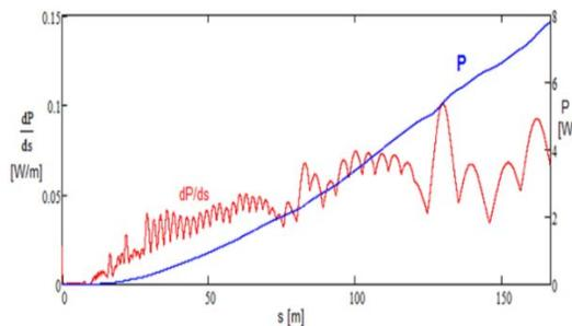
Figure 7: Beam power loss per unit length due to intra-beam stripping (red) and its integrated value along the linac (blue) for CW beam current of 2 mA.
