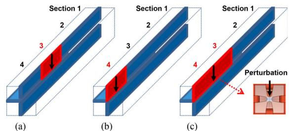
Figure 6: Three types of single vane perturbation (a) Case 1 with vane 3 movement only, (b) Case 2 with vane 4 only, and (c) Case 3 with vanes 3 and 4.
