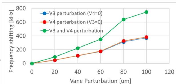
Figure 10: Frequency shift with vane distortions in RF simulation for new RFQ.
