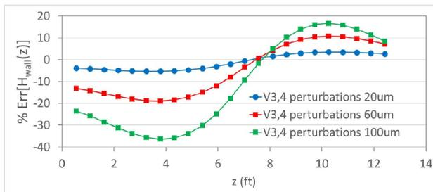
Figure 9: Field errors on the wall with movements of vanes 3 and 4 in the RFQ with end-wall rods.
