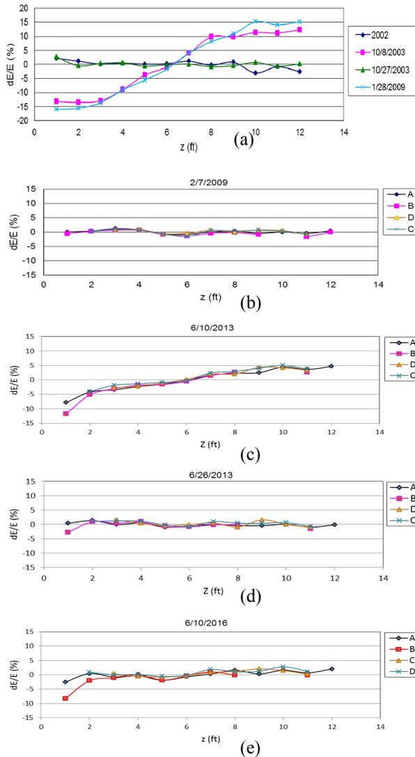
Figure 3: Measured RFQ field flatness errors in four quadrants over years of operation. (a) detuning events until 2009 shown with average of the fields in four quadrants, (b) retuned fields in 2009, (c) tilted field found in 2013 with unknown reason, (d) field error retuned for the field flatness, (e) latest measurement with a slight tilt.
