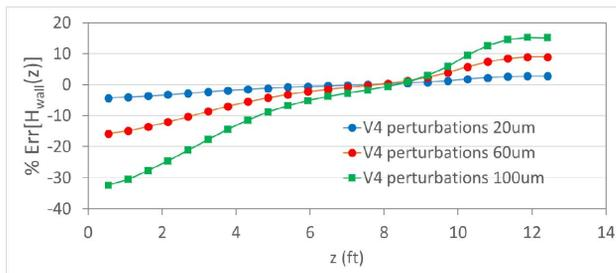
Figure 8: Field errors on the wall only with vane 4 movement in the RFQ with end-wall rods.
