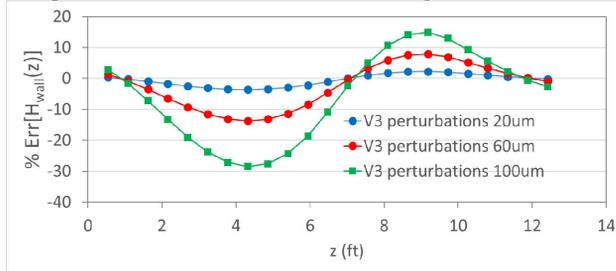
Figure 7: Field errors along the structure on the wall only with vane 3 movement in the RFQ with end-wall rods.
