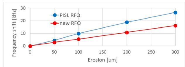
Figure 5: Frequency shifted with simulated erosion at the vane ends in low energy entrance of the RFQ stabilized with PISL and the new RFQ stabilized with end-wall rods.
