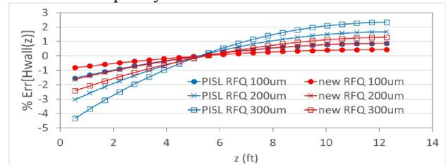
Figure 4: Fields with simulated erosion (100um - 300um) at the vane ends in low energy entrance of the RFQ stabilized with PISL and the RFQ stabilized with end-wall rods.
