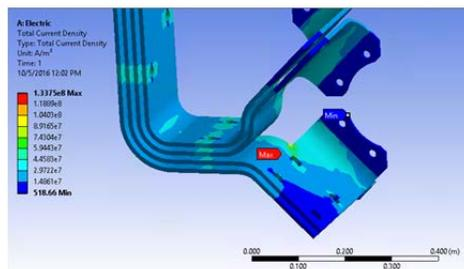
Figure 6: The current density simulation of the flag plate of 400-kW high-current stripline using (half symmetry) using ANSYS Electric.
