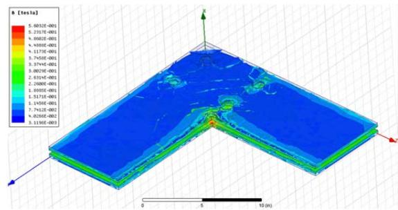
Figure 10: ANSYS Maxwell 3D result for magnetic field map of flag plate of 400-kW design each carrying 50-kA, DC in the opposite direction (+ -).
