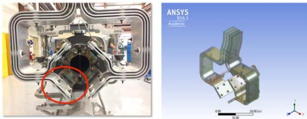
Figure 2: The 400-kW high-current stripline for NuMI.
