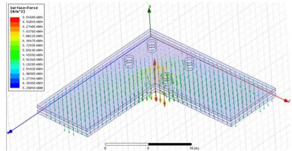
Figure 11: ANSYS Maxwell 3D result for the pressure distribution of flag plate of 400-kW design each carrying 50-kA, DC in the opposite direction (+ -).
