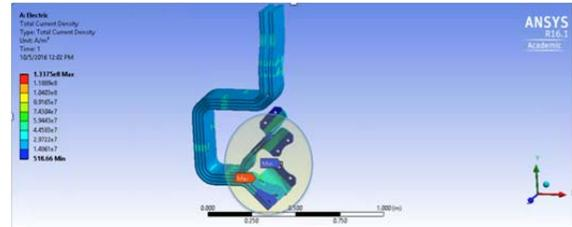
Figure 5: The current density simulation of 400-kW, high-current stripline using (half symmetry) using ANSYS Electric.
