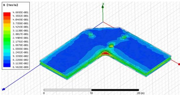
Figure 8: ANSYS Maxwell 3D result for magnetic field map of flag plate of 700-kW design each carrying 50-kA, DC in the opposite direction (+ -).
