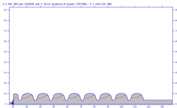
Figure 6: The design geometry of the cathode and gun structures together and the results at 2.6 GHz as calculated using SUPERFISH.
