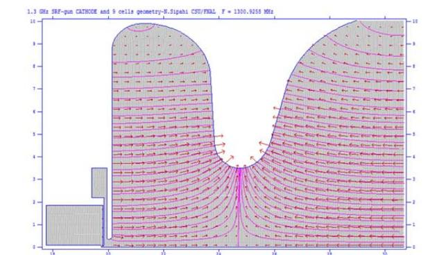
Figure 5: The magnified view of the cathode and first cell connection as shown in Figure 4 as calculated using SUPERFISH.
