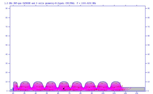
Figure 4: The design geometry of the combined structures at 1.3 GHz using SUPERFISH.
