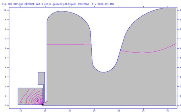
Figure 7: The magnified view of the cathode and first cell connection as shown in Figure 6 as calculated using SUPERFISH.
