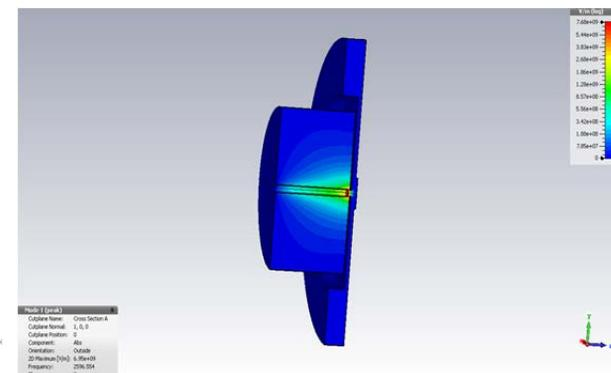
Figure 3: The cathode geometry design with the frequency matched to 2.6 GHz and the contour plot of fields all generated in CST MWS.
