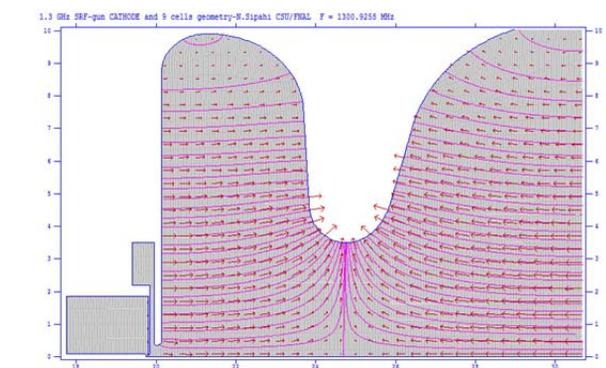
Figure 5: The magnified view of the cathode and first cell connection as shown in Figure 4 as calculated using SUPERFISH.
