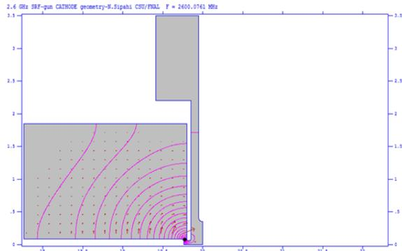
Figure 2: The cathode design geometry at 2.6 GHz with the field distribution using SUPERFISH.
