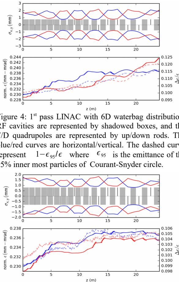
Figure 4: 1<sup>st</sup> pass LINAC with 6D waterbag distribution. RF cavities are represented by shadowed boxes, and the F/D quadrupoles are represented by up/down rods. The blue/red curves are horizontal/vertical. The dashed curve represent  $1 - \epsilon_{95}/\epsilon$  where  $\epsilon_{95}$  is the emittance of the 95% inner most particles of Courant-Snyder circle.
