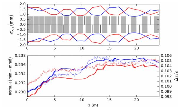
Figure 5: 2<sup>nd</sup> pass LINAC with 6D waterbag distribution.
