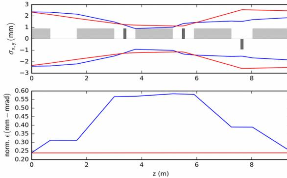
Figure 8: Transverse beam at the 1<sup>st</sup> arc. Bending magnets are represented by shaded boxes.
