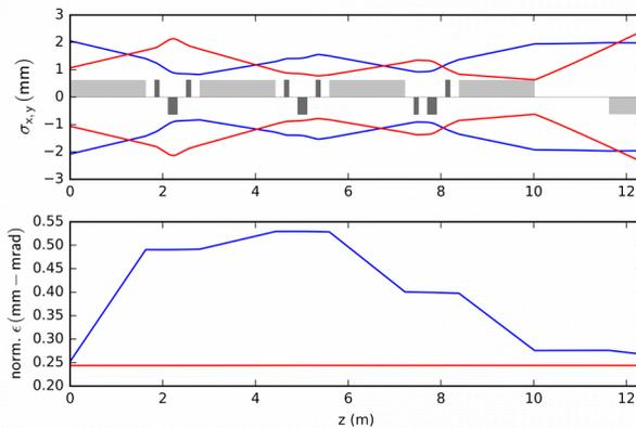
Figure 9: Transverse beam at the 2<sup>nd</sup> arc. The downward shaded box represent negative angle bending magnet.
