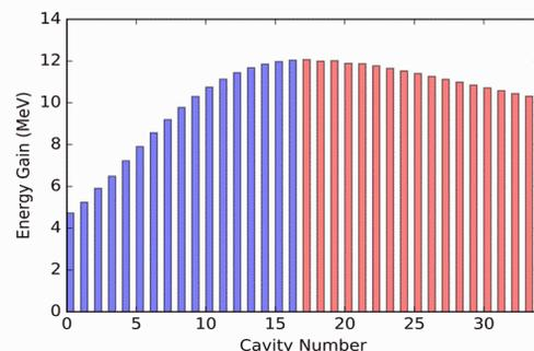
Figure 2: Energy gain of each cavities.
