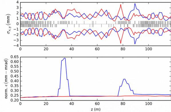
Figure 10: Transverse beam envelope from the 1<sup>st</sup> pass LINAC entrance to 2<sup>nd</sup> pass LINAC exit.
