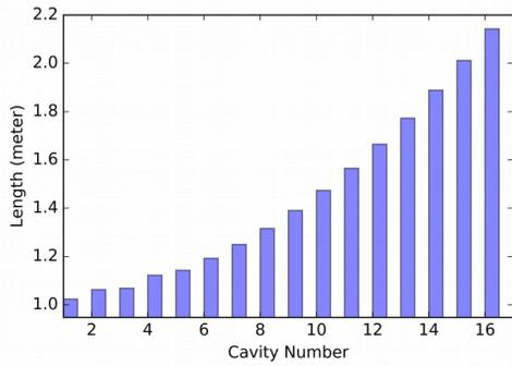
Figure 3: Separation length from the  $i$ -th cavity entrance to the next cavity entrance.
