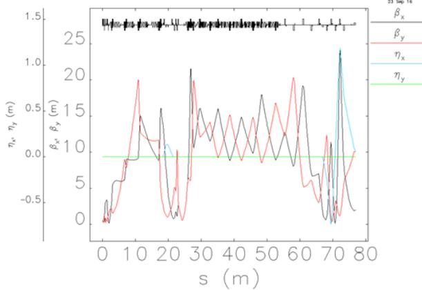
Figure 2: Lattice functions for APS injector linac for beam injection into the PAR.
