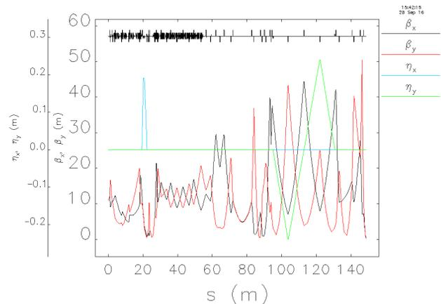
Figure 3: Lattice functions along APS LINAC and LEA optimized for PCG.
